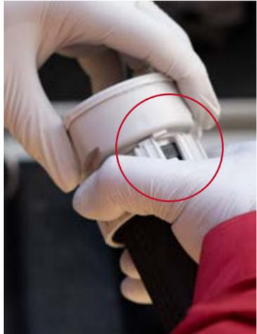
2. Connect the Reporter (Top) to the Detector (Bottom). For the device to work properly you must
