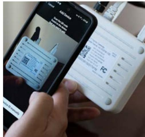
5. Scan the QR code on the bottom of the Encircle Gateway, or manually enter the entire EUI code starting with the "eui-" characters
