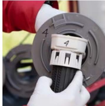
2. Using a permanent marker, write the same numbers on the Encircle Stations that were written on the Encircle Smart Sensors
