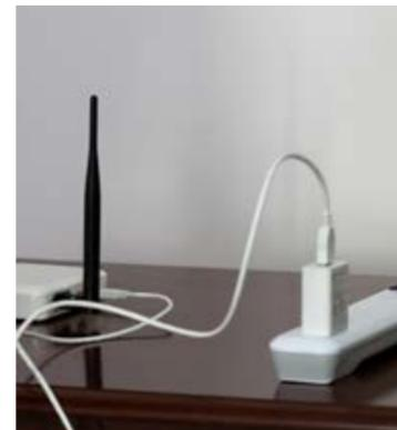
3. Connect the power cable into the Encircle Gateway and plug into an available power outlet.
