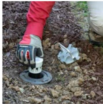
3. Insert the corresponding Encircle Smart Sensor inside the Encircle Station (labels must match)
