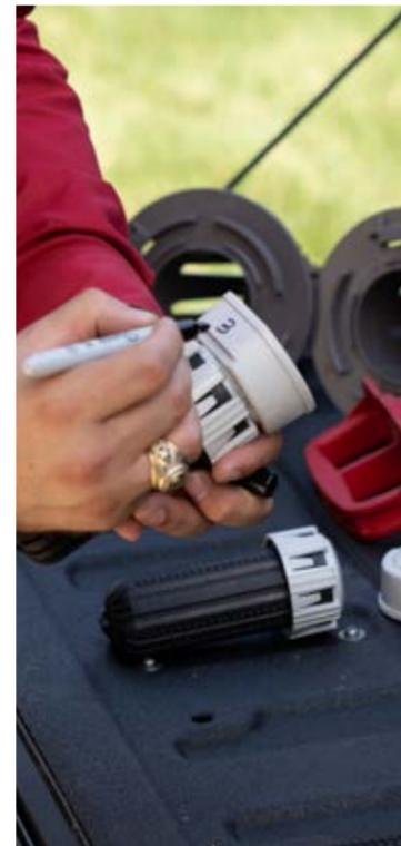
9. Using a permanent marker, write the nickname on the Reporter (e.g., 01, 02, 03, etc.)
