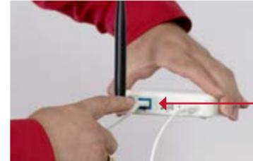
2. Plug one end of the ethernet cable into the Encircle Gateway and the other end into an available port on the customer's Internet router.
