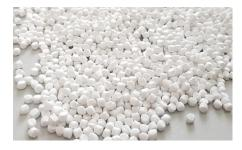
Containers are processed into resin pellets to be used in manufacturing other products.
